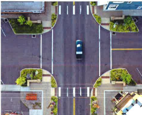
Bulb outs increase curb radii
