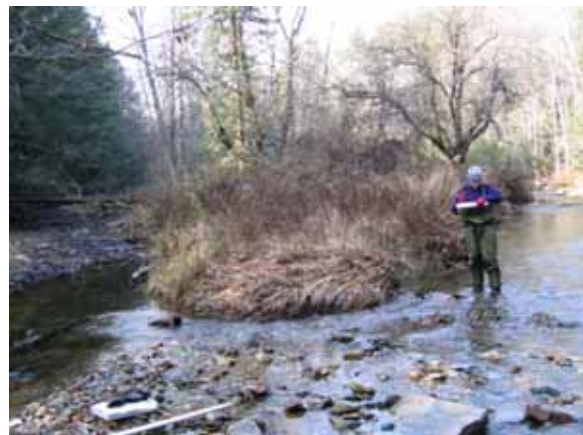
Figure 5.67: Lower end of large channel avulsion with active flood chute near intersection of Smith Hill Road and Stony Brook Road
